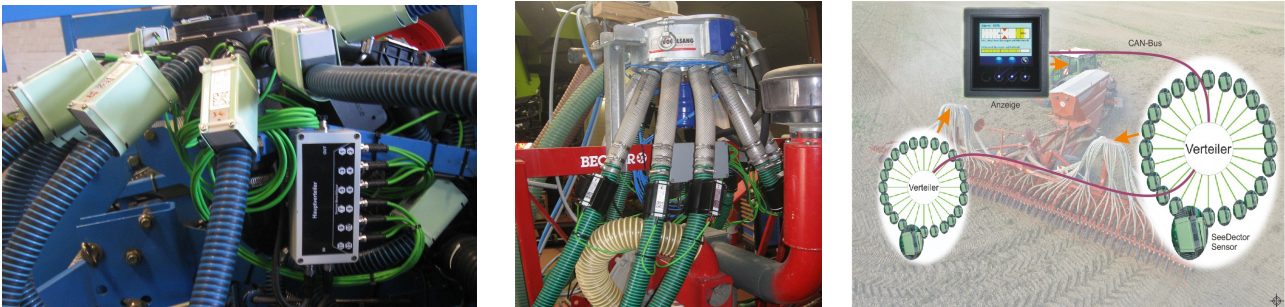
Fig. 5: MSO SeeDector Sensors and Hub on a seed drill (left), on a slurry distribution head (mid), Integration in the MSO SeedMon System for Blockage Monitoring (right) [5]
