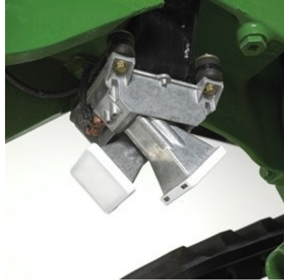
Fig. 3: Radar speed sensors in Janus Configuration, left: MSO SpeedWedge, right: John Deere Radar Sensor; Corporate photographs
