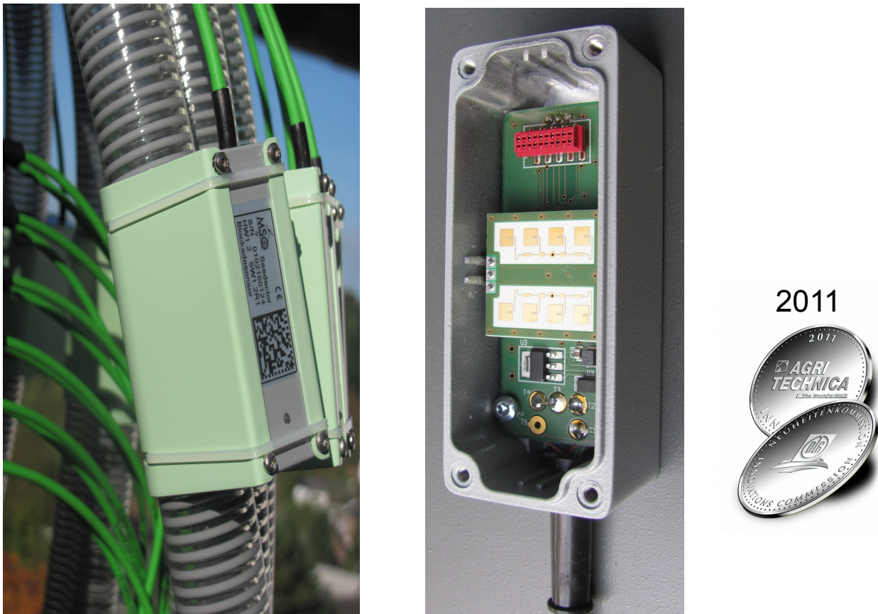
Fig. 4: MSO SeeDector Sensor mounted (left); MSO SeeDector Sensor opened (mid); Silver medal award for MSO from the DLG novelties commission at Agritechnica 2011 (right); Corporate Photographs MSO
