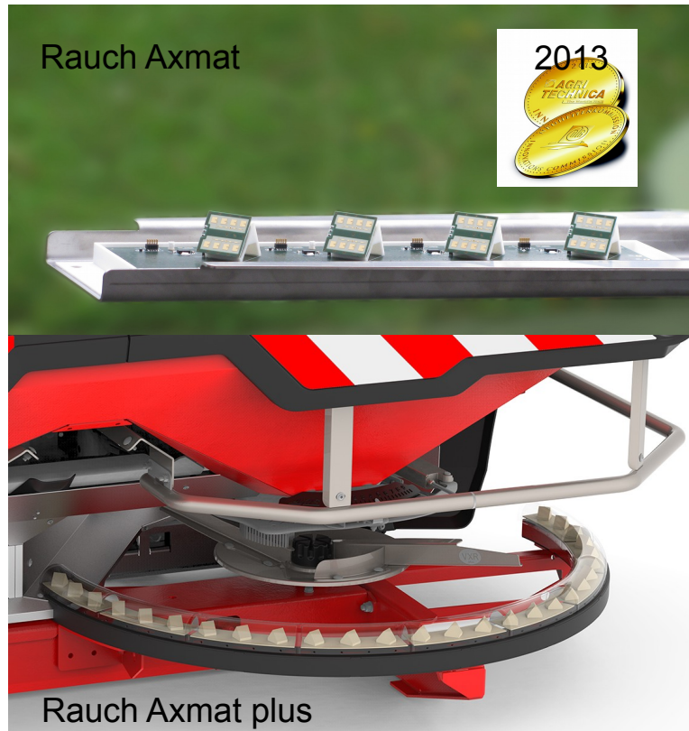
Fig. 6: Rauch Axmat picture above : Swivel arm system for detection of lateral material distribution on a disc spreader (Corporate photograph MSO); below : Rauch Axmat plus as a stationary ring-segment with 27 Radar Sensors (Press-Release Photograph Rauch)
