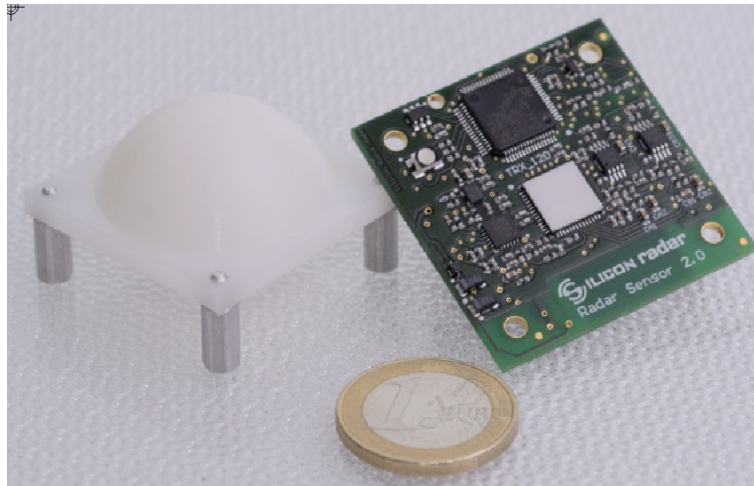
Fig. 12: Evaluation Kit for a 120 GHz FMCW Radar from Silicon Radar [11] with dielectric lens.
